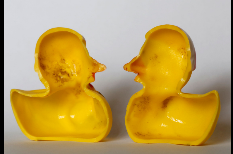
Rubber duckie cut in half to show inconsistent wall thickness.
