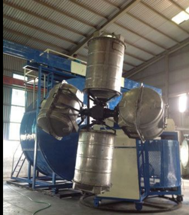
A large rotomolding machine used for making 50 gallon barrels.
