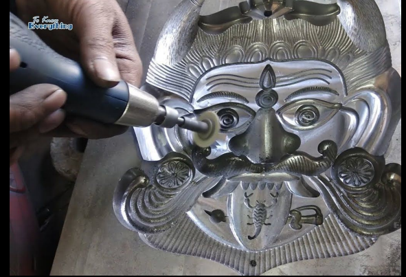
An Injection Mold being polished.
