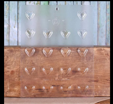
Thin, clear plastic - clamshell packaging (below) candy molds made through vacuum forming
