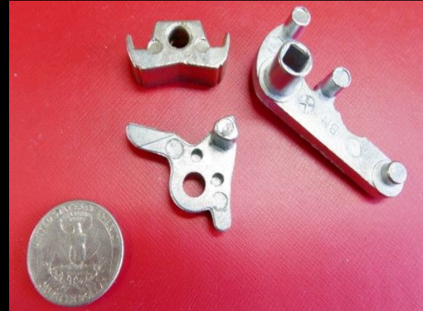
Circular ejector pin marks.
