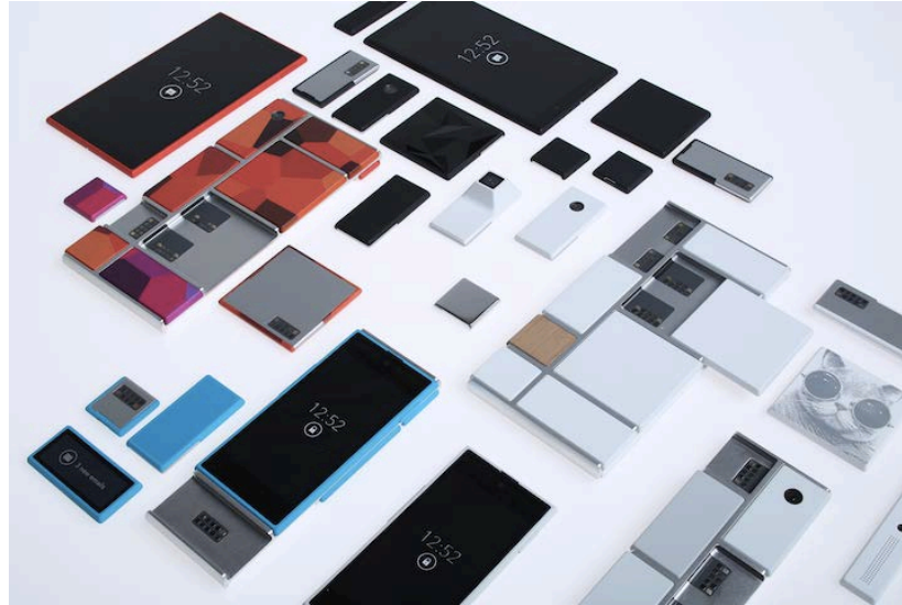
Reconfigurable, modular mobile device
